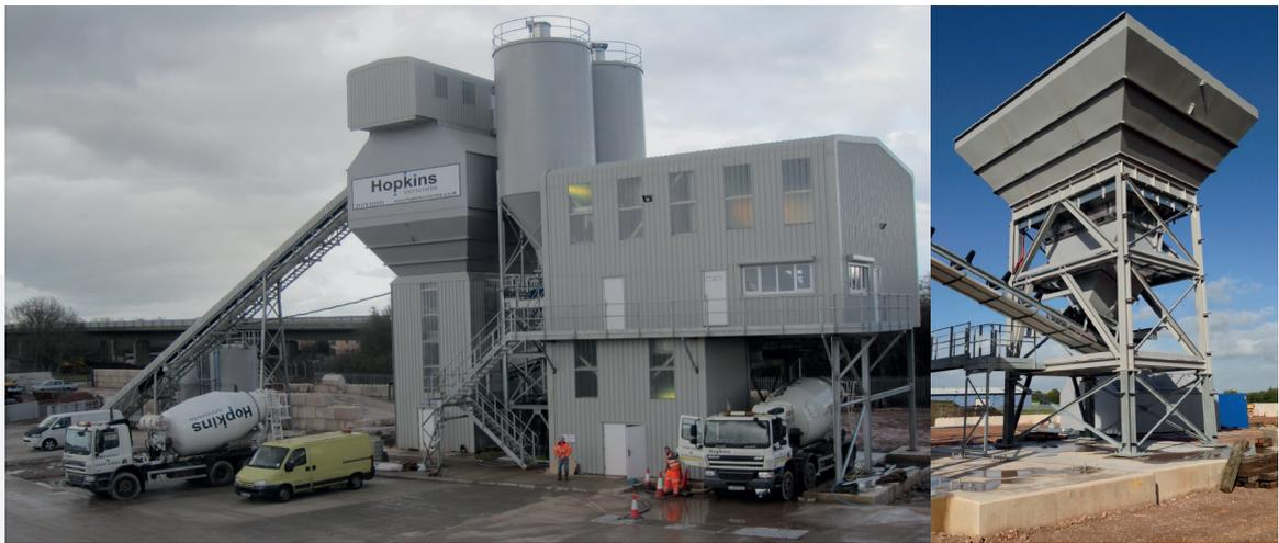
**We manufactured a high output (160m<sup>3</sup> per hour) batching plant for Hopkins Concrete, designed to suit our client's site and requirements**
